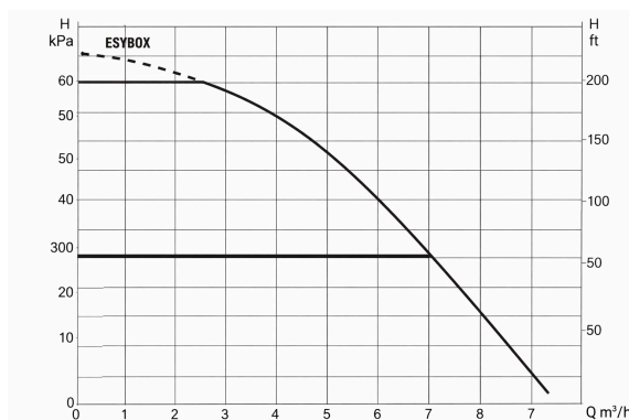
Manufacturer's pump curve — head (H) vs flow (Q). Flow @ 3 bar (~30m head) ≈ 80 L/min.
