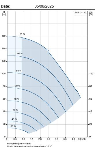
Liquid temperature during operation = 20 °C Density = 998.2 kg/m<sup>3</sup>
