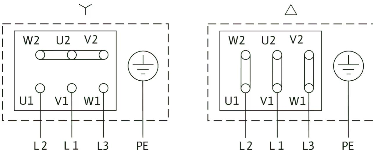
Δ: Connection diagram delta connection
