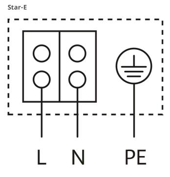
Blocking current-proof motor **Single-phase motor** (EM) 2-pole - 1~230 V, 50 Hz With built-in capacitor
