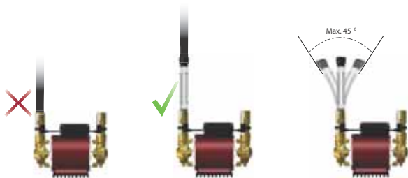
Fig. 18 Connecting the flexible hoses
