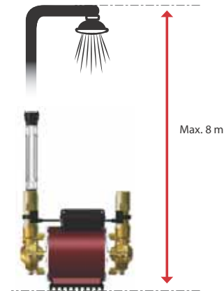
Fig. 33 Maximum static head
