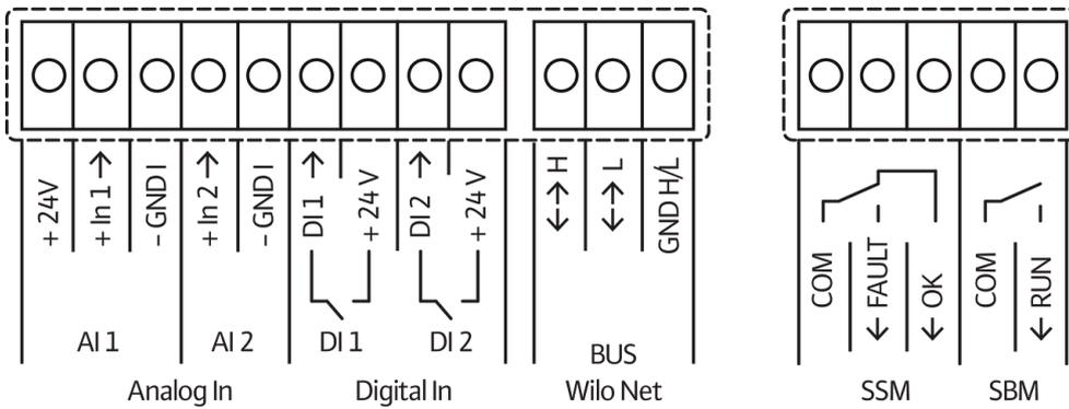
SSM: Collective fault signal (NC contact in accordance with VDI 3814, load capacity 1 A, 250 V ~)
