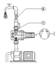
It is recommended to connect the output of the device to the system by means of a ball valve and flexible tube (fig. B).
