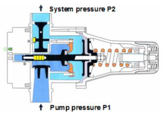
When the pump has stopped, the chambers do not communicate as the diffuser is closed due to the pressure in the primary chamber being higher than that of the secondary chamber.
