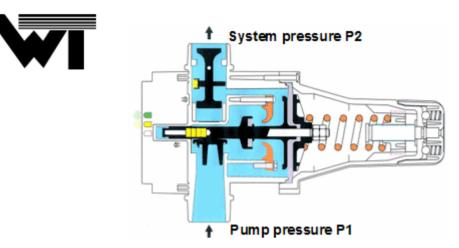
When the pump is operating, the chambers communicate as the diffuser is more or less open due to the fact that a pressure differential is created between the primary chamber and the secondary chamber depending on the adjustment.
