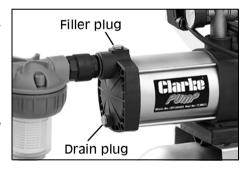
NOTE: If a filter is fitted to your pump it is recommended that you remove the brass plug on top and fill the filter bowl with water.
