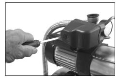
These pressures are factory set but can be adjusted using the plastic screw on the pressure switch. The pump may continue to operate for a short while after the supply valve is turned off until the cut-out pressure is reached.
