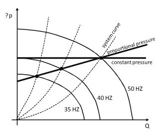
Constant differential pressure control can be extended to the operation in a group, i.e. twin pumps application.
