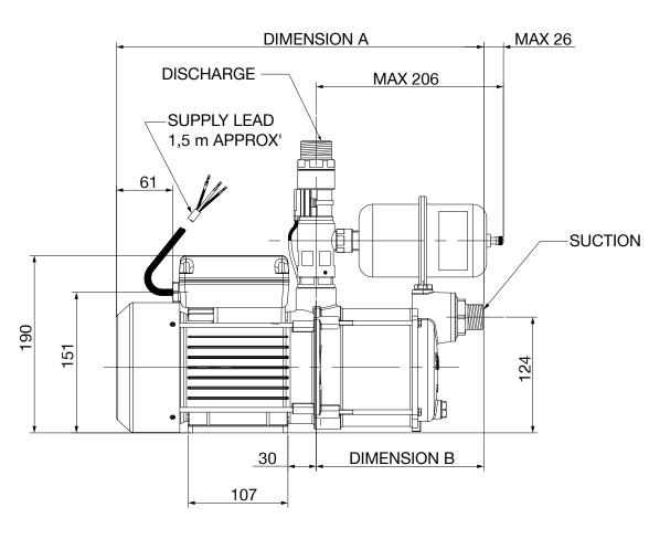
Note: The pressure vessel can be re-positioned if required to suit specific installations. However care must be taken when re-positioning to ensure no strain is placed upon the pressure switch or flow switch cables (not shown).
