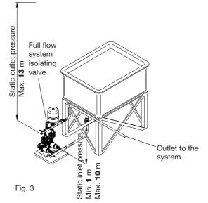
3.11 **The cold water supply: Must be a DEDICATED AIR FREE** supply via a tank connector and must be able to self vent. Flexible hoses are supplied with the pump set and must be fitted between both suction and delivery manifolds and the installation pipework.
