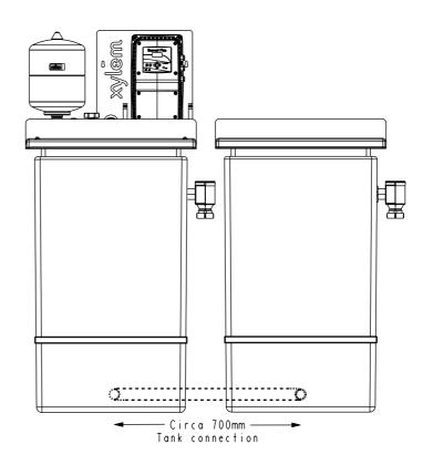
For applications which require a larger storage capacity, a 250 litre Assist tank can be purchased and installed alongside the Resvari Plus. This takes the total nominal volume of the unit up to 500 litres, perfect for sustained high volume requirement such as schools and sports Halls, where water is required for longer periods of time compared to a traditional domestic dwelling.
