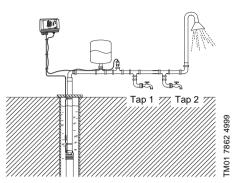
In fig. 7, tap 1 is placed close to the pressure sensor. Therefore, the pressure will be kept nearly constant at tap 1, as the friction loss is small. At the shower and tap 2, the friction loss is bigger. This, of course, depends on the piping. However, old and furred-up piping may cause inconvenience due to friction loss.
