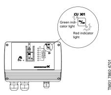
The green and red indicator lights in the on/off button indicate pump operating condition as follows:
