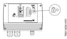
When the buttons are locked, the indicator light is permanently on, see fig. 11.
