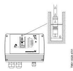
The indication of pump operation can be changed by means of the R100.
