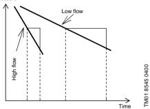
**Note:** When the pressure is dropping 0.1 bar/s or faster, the pump will start immediately.
