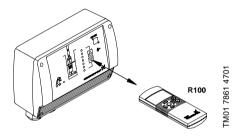
The R100 offers possibilities of setting and status displays for the CU 301.
