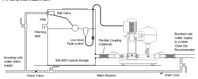
Any bypass arrangement must be installed strictly in accordance with the Water Byelaws Regulations. The bypass should be drained when not in use to prevent stagnation. The diagram above is for guidance only.
