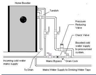
2. The unit should be installed on a solid flat surface to adequately support the weight of the water tank, and to help reduce noise/ vibration.
