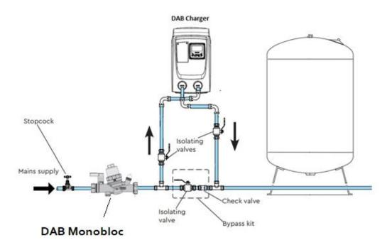
The DAB Monobloc should be installed between the stock cock and system. Before any outlets, taps or pump.
