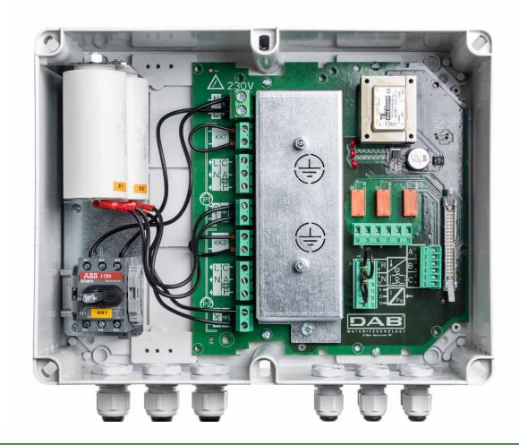
**e.box basic** is an electronic control panel for the protection and automatic operation of one or two electronic submersible pumps or single-phase pressurization for domestic applications. The **e.box** panel is compatible with all models of pumps with current between 1 and 12 A with power up to 2.2Kw as reported by the products compatibility chart.
