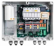
**e.box plus** is an electronic control panel for the protection and automatic operation of one or two submersible pumps or pressurizing both single-phase and three-phase, installed in domestic, civil and industrial environments. Thanks to the possibility of adjusting the current, **e.box** is compatible with all models of pumps with a current between 1 and 12A with power up to 5.5Kw as reported by the products compatibility chart.
