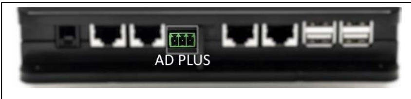
Figure 9A - Connector position in the AD plus and DConnect box, e.g. can-bus straight cable connection, connector name DConnect box for connection with AD plus
