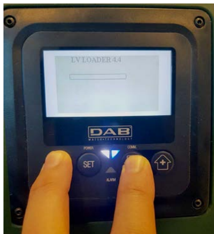
Figure 9C - Loader access for e.sybox mini3 Sw 1.X update
