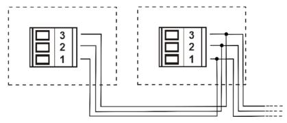
Figure 4: Connection of the multi-inverter communication
