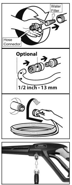
7. Connect the spray lance to the gun assembly and tighten securely by turning the locking rina.
