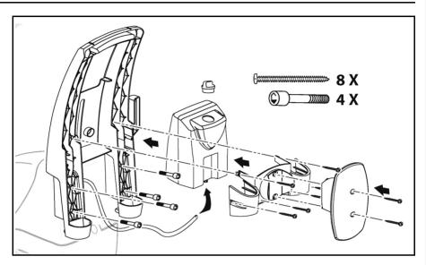
1. Fit the handle first then the detergent tank, followed by the tool holder and finally the hose hook to the hot washer as shown above using the 4 bolts (for the handle) and screws (for the tool holder, hose hook) supplied.
