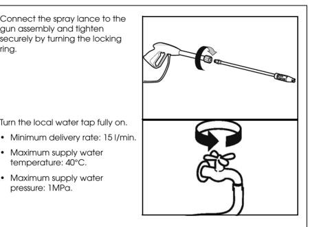
WARNING: THE HOT WASHER CAN ONLY BE CONNECTED TO THE WATER MAINS IF SEPARATED BY A BACKFLOW PREVENTER. MAKE SURE THAT THE HOSE IS AT LEAST 13MM-1/2 INCH IN DIAMETER AND IS REINFORCED.
