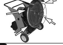
3. Fit the handle to the rear of the heater using four bolts/nuts supplied loose.
