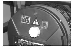
Turn the temperature control knob to adjust the target temperature required. This setting will be shown by the digital display.
