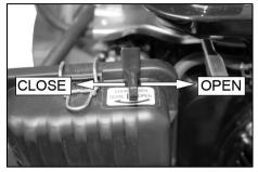
3. Set the fuel supply valve to the ON position.
