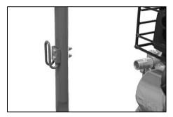
Slide the bottle holder over the bracket and place the bottle in the holder.
