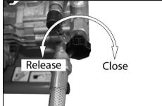
9. Turn the self-suction valve to the on position.
