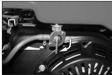
4. Slide the throttle lever to the left approximately 3/4 of the way.
