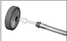
3. Remove the water inlet filter.
