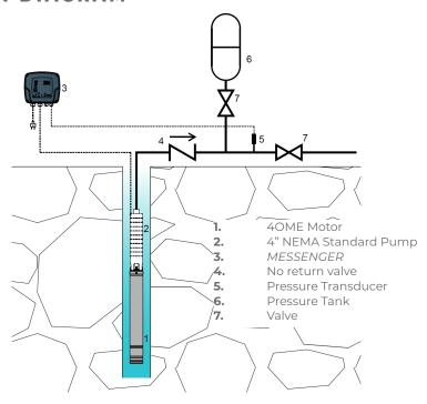
As you can see in the above connection diagram, hydraulic system is considerably simplified too. Indeed you just need to install a small pressure tank and a no return valve in order to keep the plant full of water.
