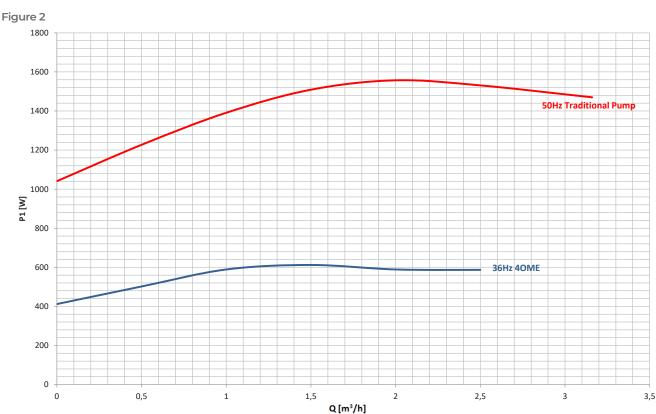
As you can see in the first diagram (Figure 1), the red curve represents a traditional 50Hz pump connected to standard motor without inverter. The blue area is the whole area of use of the same pump connected to the submersible 40ME motor, having 15 - 55Hz as operating range.
