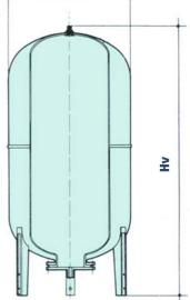
Pressure vessels are available in a range of sizes from 5 L. The vertical series have a control panel mounting bracket. All vessels incorporate a replaceable rubber membrane which are suitable for temperatures from 0 to 99°C.
