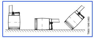
Pumps with vertical level switch must be used in vertical position.
