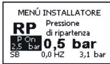
Figure 13: Setting the restart pressure
