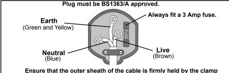
Elistife that the outer sheath of the cable is lifting field by the clamp
