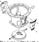
The pump is fitted with a balanced O-ring seal unit with a rigid torque-transmission system. This seal type is assembled in a cartridge unit which makes replacement safe and easy. Due to the balancing, this seal type is suitable for high-pressure applications. The cartridge construction also protects the pump shaft from possible wear from a dynamic O-ring between pump shaft and shaft seal.
