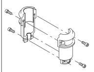
The motor stool connects the pump head and motor. The pump head has a combined 1/2" priming plug and vent screw.
