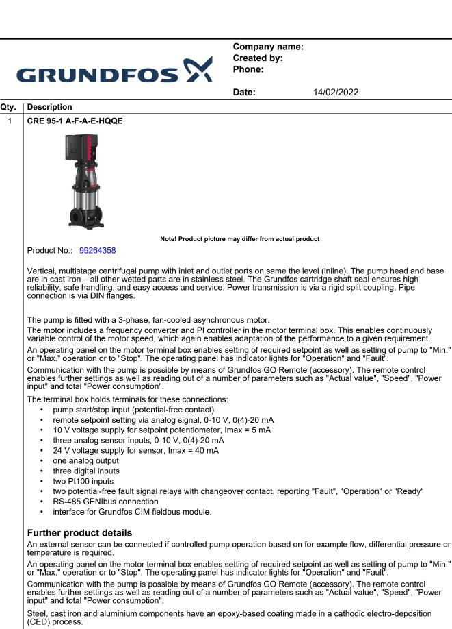
CED is a high-quality dip-painting process where an electrical field around the products ensures deposition of paint particles as a thin, well-controlled layer on the surface.
