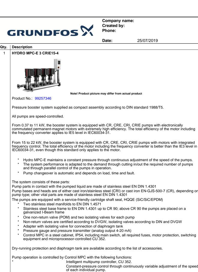
Pump bases and heads are of either cast iron/stainless steel (CRI) or cast iron EN-GJS-500-7 (CR), depending on Stainless steel base frame to EN DIN 1.4301 up to CR 90; above CR 90 the pumps are placed on a Non-return valves are certified according to DVGW, isolating valves according to DIN and DVGW Control MPC in a steel cabinet, IP54, including main switch, all required fuses, motor protection, switching
