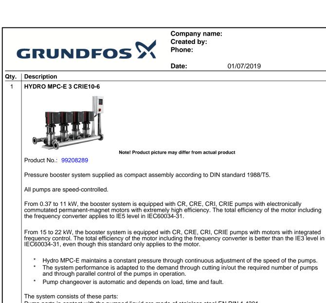
Pump parts in contact with the pumped liquid are made of stainless steel EN DIN 1.4301 Pump bases and heads are of either cast iron/stainless steel (CRI) or cast iron EN-GJS-500-7 (CR), depending on pump type; other vital parts are made of stainless steel EN DIN 1.4301
