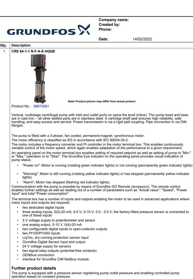
An operating panel on the motor terminal box enables setting of required setpoint as well as setting of pump to "Min." or "Max." operation or to "Stop". The Grundfos Eye indicator on the operating panel provides visual indication of pump status:
