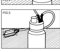
When the float switch reaches the minimum level it will automatically switch the pump off.
