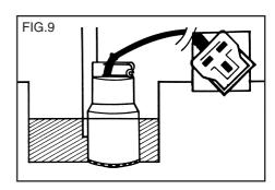
When submersing or lifting the pump it will be necessary to use a rope or chain, this must be attached to the transport handle.
