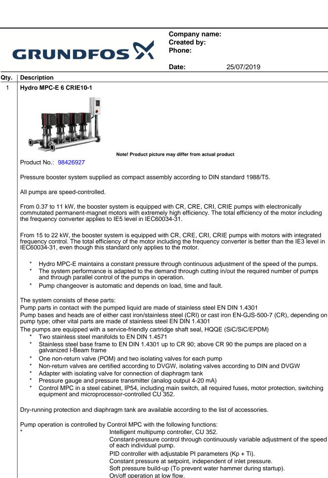
Automatic cascade control of pumps for optimum efficiency.
