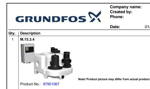
Supplied as complete unit ready for installation, the Multilift consist of a fully integrated collecting tank with pump and submersible motor, non-return valve, discharge adapter with flexible connection piece DN100 mounted on the collecting tank and a pre-wired Controller incl. a level sensor.
