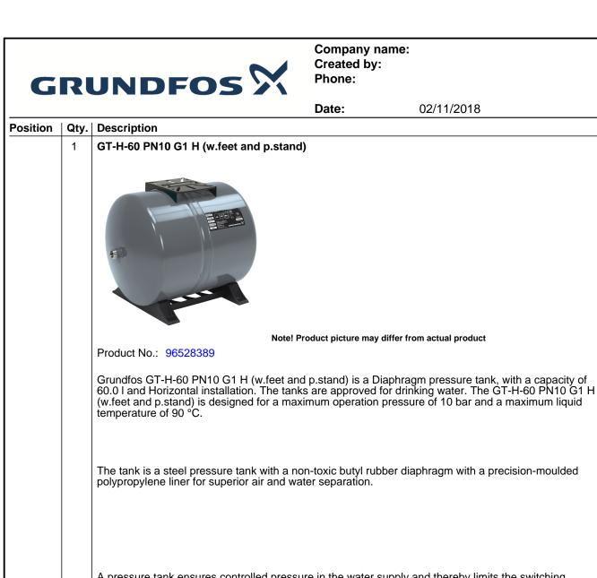
A pressure tank ensures controlled pressure in the water supply and thereby limits the switching frequency of the pump in case of low water consumption or leakage loss. The result is increased comfort in your installation by limiting the start/stop frequency of your pump, and it increases system comfort by compensating for pressure drops when a tap is opened, while reducing problems with water hammer in the pipework.
