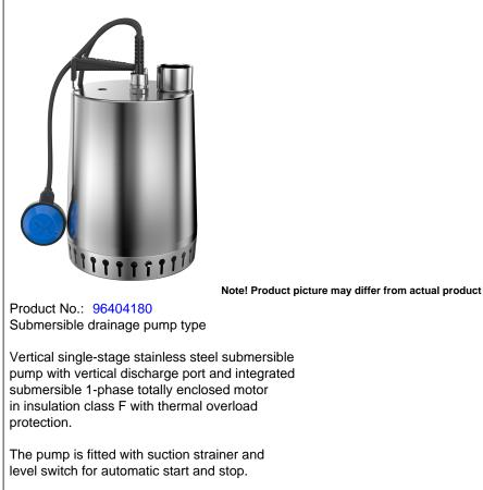
The impeller is a SEMI OPEN impeller for 12 mm free passage suitable for pumping groundwater, surface water, rain water and similar.
