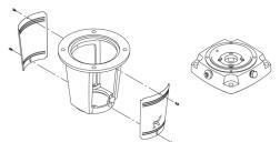
The pump is fitted with a balanced O-ring seal unit with a rigid torque-transmission system. This seal type is assembled in a cartridge unit which makes replacement safe and easy. Due to the balancing, this seal type is suitable for high-pressure applications. The cartridge construction also protects the pump shaft from possible wear from a dynamic O-ring between pump shaft and shaft seal.
