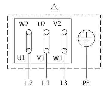
Δ: Connection diagram delta connection
