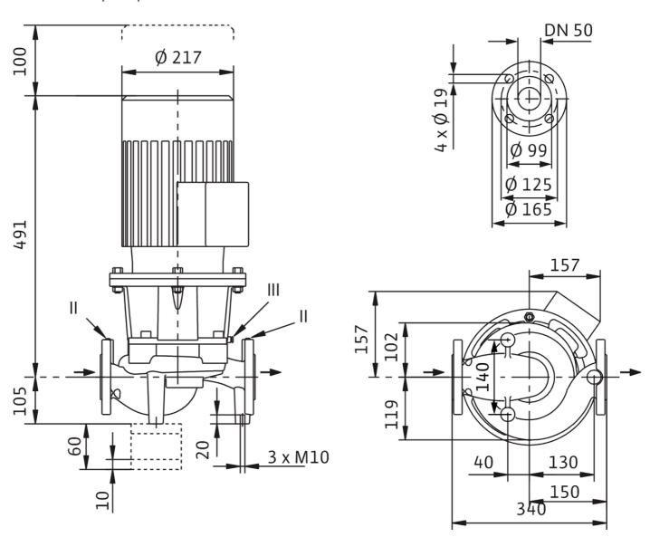
II Pressure measuring connection  $R^1/_8$ ; III Ventilation  $R^1/_8$
