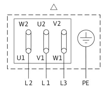
Δ: Connection diagram delta connection
