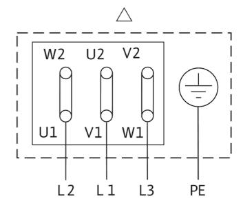
Δ: Connection diagram delta connection
