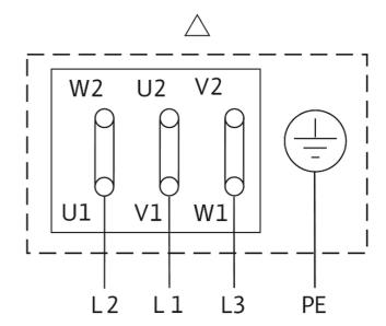
Δ: Connection diagram delta connection
