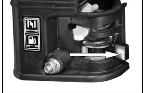
2. To start a cold engine, move the choke lever to the 'OFF' position.
